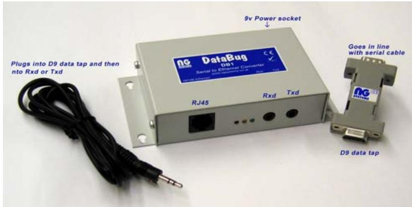
The D9 data tap is placed in line between the two serial devices. The 3.5 mm stereo cable is connected to the D9 data tap and then into the Rxd or the Txd socket on the DataBug.
